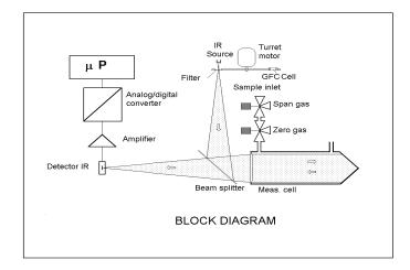
A wide band infrared radiation is emitted by a non metallic, high stability source.
