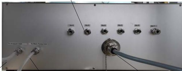
Multi point gas inlets
